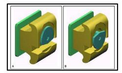
Figure 4: Mobil-lock (A) Opened (B) Closed
