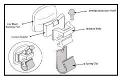
Figure 5: Parts of Speed Bracket
