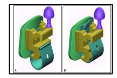
**Figure 6:** Speed Bracket (A) Opened (B) Closed positions
