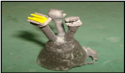
Figure 4. Casting Of Metal Housing and Attachment Of Hader Clip
